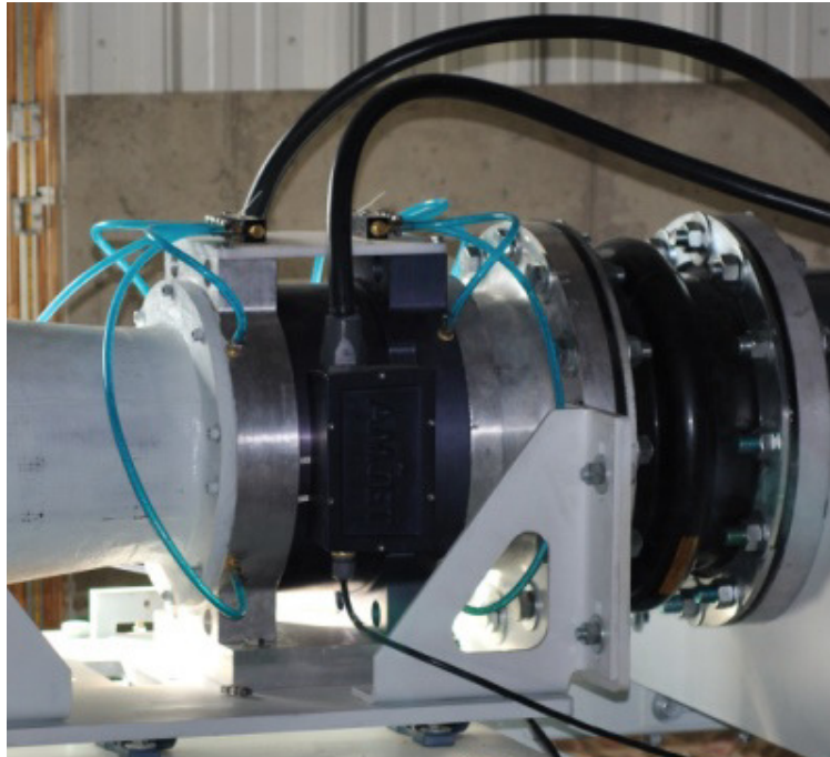
ATS-8 turbine/generator with 8 inch internal diameter
