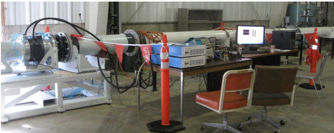
FIG. 2 Test stand at the University of Iowa, 1/8-scale unit on the left (cables); instrumentation and monitor on the right.
